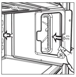
When reassembling the catalytic side liners, ensure they sit correctly.
